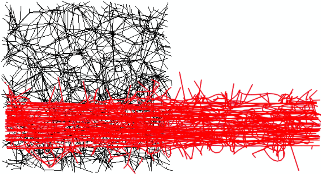
Fig. 3. Deformed network configuration (red) corresponding to an axial stretch of 1.92. The undeformed configuration is shown (black) for reference.
